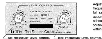
Adjusts the sound level of the mid and high frequencies when driving the speaker system as a full range speaker system. Make the level setting according to the environmental conditions, although almost flat frequency response is obtainable so far as the level controls remain within the "NORMAL" ranges.
