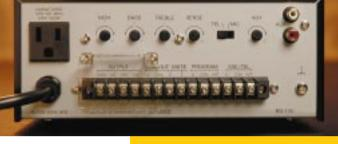
Simple layout makes set-up easy—even for inexperienced technicians. Short-circuit protection and speaker terminal covers offer added security and help assure reliability in demanding environments.
