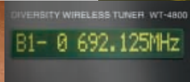
The Password receiver features an on-board scanner and an LCD for RF and AF metering, as well as frequency setting.
