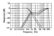
\_\_\_\_\_System selection: Install between terminal Nos. 3 and 4 ......System selection: Jumper not installed Note that the three identical curves indicate +2, 0 and -2 settings
