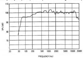
Measured at 1 watt(at 200Hz) and 2 meters. SPL shows the converted level into 1W/1m.
