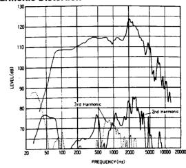
Measured at 30 watts (-10dB power), 1 meter.
