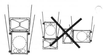
Make sure to suspend the constant directivity horn to upper direction.
